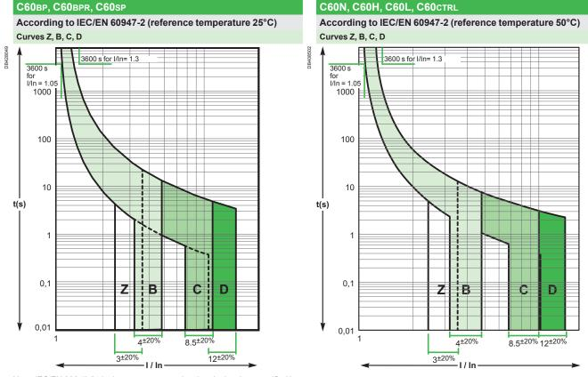
Note: IEC/EN 60947-2 tripping curves, respecting the tripping time specified by the standards UL 489, CSA C22.2 No 5, UL 1077 and CSA C22.2 No 235
