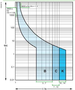
Note: IEC/EN 60947-2 tripping curves, respecting the tripping time specified by the standards UL 1077 and CSA C22.2 No 235
