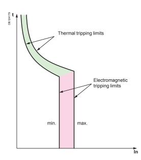
The following curves show the total fault current breaking time, depending on its amperage. For example: based on the curve on "Circuit breakers tripping curves", page 86, a C60 circuit breaker of curve C, 20 A rating, will interrupt a current of 100 A (5 times the rated current In) in:
